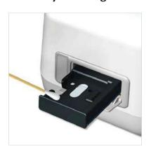
The blood, moisture or dust that enters the tray may lead to failure of the Sampinute<sup>TM</sup> Analyzer. Wipe the tray carefully with an alcohol-moistened swab if needed.
