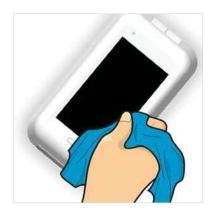
Clean the analyzer periodically with a soft and dry cloth. Do not use highly corrosive cleaning solution or chemicals, or a cleaning tissue contains chemical substances that may damage the device.
